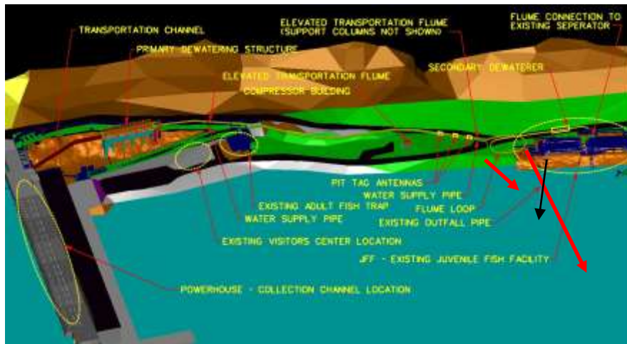
Figure A. Depiction of overall Lower Granite Dam JBS Phase 1 upgrade. Bright red lines in tailrace indicates location of new primary and emergency bypass outfalls.
